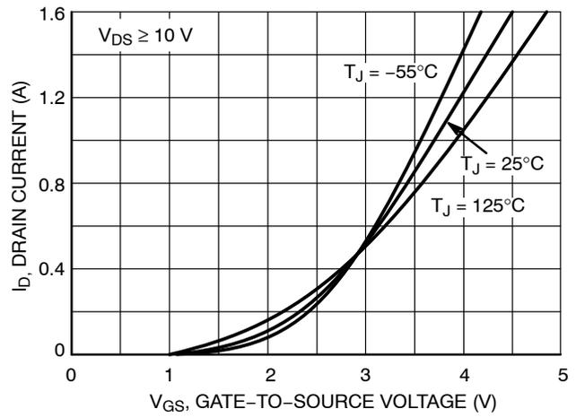
Figure 2. Transfer Characteristics
