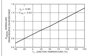
Figure 3. On-Resistance Variation with Temperature.
