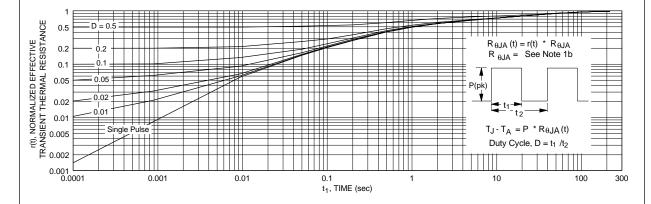
Figure 17. Transient Thermal Response Curve.
