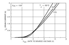
Figure 5. Transfer Characteristics.
