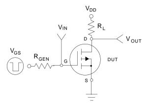
Figure 11. Switching Test Circuit.
