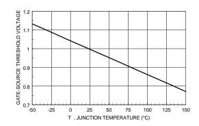
Figure 6. Gate Threshold Variation with Temperature.
