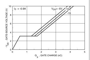
Figure 10. Gate Charge Characteristics.
