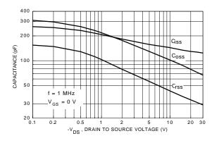
Figure 9. Capacitance Characteristics.
