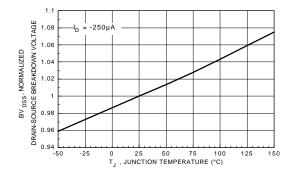
Figure 7. Breakdown Voltage Variation with Temperature.
