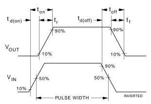
Figure 12. Switching Waveforms.
